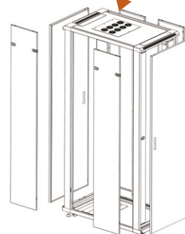
door and side panel. 4. Assemble front/rear
